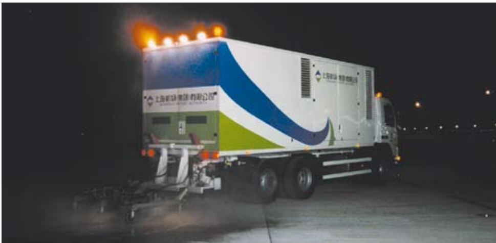
Runway Cleaner for the removal of rubber deposits from airport runways.
