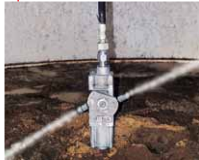
Internal vessel and tank cleaning with the tank cleaning head TankMaster® and the corresponding positioning device.
