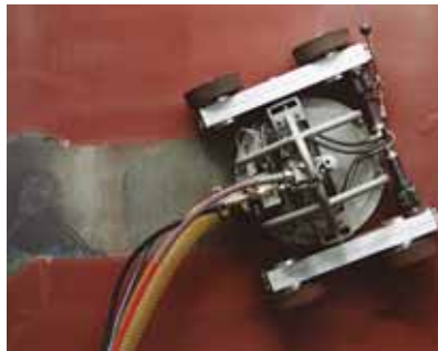
The Vacuum Lizard V2500 with remote control for emissions-free large-scale surface preparation.
