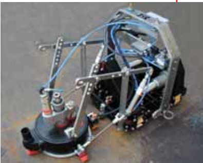
The Magnetic Lizard M2500 is a self-propelled cleaning system which is adhered onto the surface via permanent magnet.
